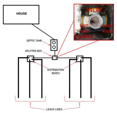
Every year, the splitter box should be alternated to divert effluent to one field, and block flow to the other, to let that field rest.
