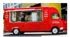
Concession Trailers and Trucks are fully self-contained units with mechanical refrigeration, a complete plumbing system including a hot water tank, and plenty of storage space for multiple day events. These are generally considered "restaurants on wheels."
