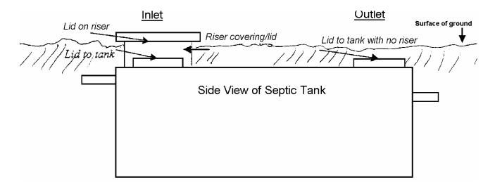
There are two openings on most septic tanks, an inlet and an outlet. One may have an extension called a riser that provided ground surface accessibility to the tank for cleaning and maintenance purposes. The other opening, more than likely, will not have a riser on it. However, please be aware that risers can be on either the inlet or the outlet side of the septic tank. The Health District will need both openings of the septic tank uncovered and accessible at the time of inspection.
